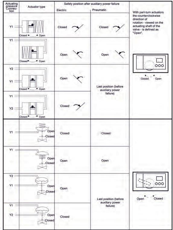
Illustration 7: Pneumatic connection positioning effect
