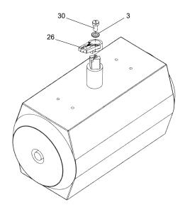
Illustration 20: Mounting the driver on the actuator
