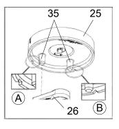
Illustration 21: Mounting the positioner on the actuator
