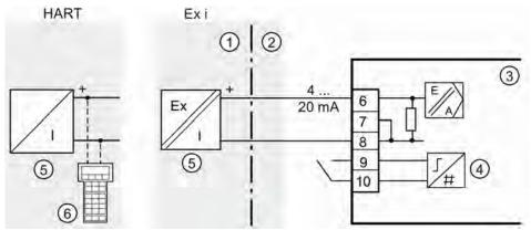
Illustration 26: 2-wire connection of 2-wire device
