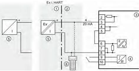
Illustration 27: 2-wire connection of 2/3/4-wire device
