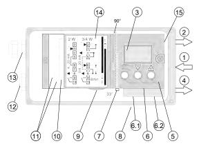
Supply air input Output: actuating pressure Y1 3 Display Output: actuating pressure Y2 \*) 4 5 **Operating Buttons** 6 Restrictor Y1 6.1 Restrictor Y1 \*) 6.2 Restrictor Y2 \*) Transmission ratio selector 8 Silencer Slip clutch adjusting wheel 10 Basic device connecting termin-Connecting terminals 11 Option modules 12 Blinding plug 13 Cable gland 14 Clamping plate for cover Purging air switch with double/acting devices
