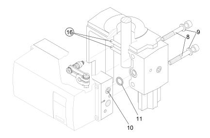
Illustration 12: Mounting the positioner on the actuator
