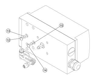
Illustration 11: Mounting the lever on the positioner
