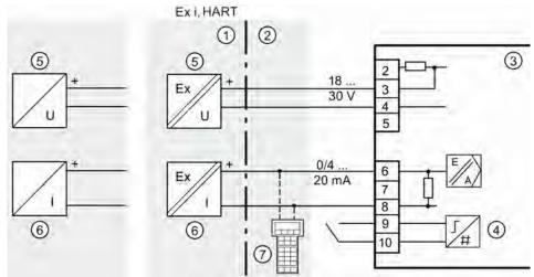
Illustration 29: 4-wire connection of 2/3/4-wire device
