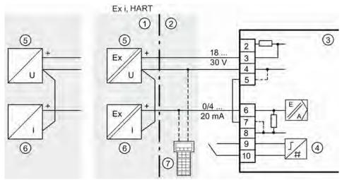
Illustration 28: 3-wire connection of 2/3/4-wire device
