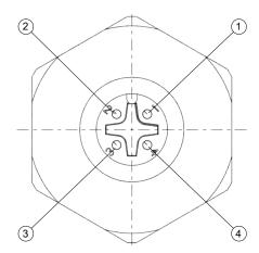
Illustration 37: Pin diagram - seen from pin side
