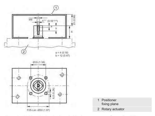
Illustration 23: Mounting bracket (supplied by the actuator manufacturer) and dimensions
