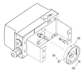
Illustration 19: Mounting the coupling wheel on the positioner
